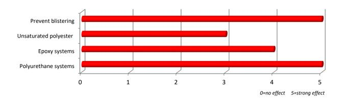
**LNIQ**<sup>®</sup> **FOAM P-599** is a strong anti-foam and air-release agent especially suitable for unsaturated polyester resin, ambient-curing plastic systems, adhesives and sealants, especially for polyurethane based resin systems. The additive furthermore helps tod avoid pinholing or popping.
